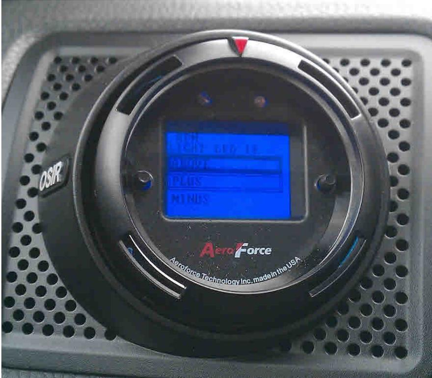
Next, enter the number by toggling right or left through the list of numbers starting with the most significant digit. Once you're on the number press both buttons, then repeat until you've entered all digits. At the end of the number list you will see a "P" and "X". Select "P" to enter a decimal point, "X" to save.
