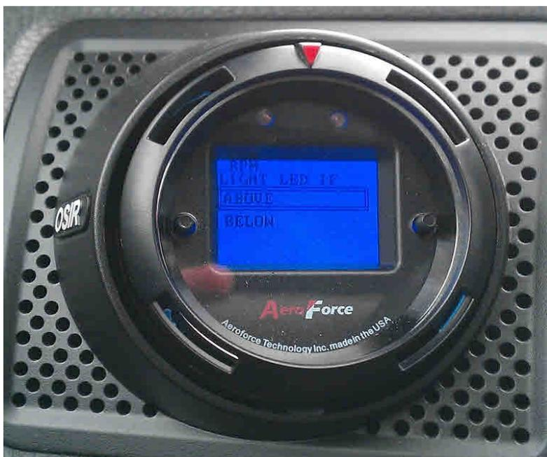
Press both buttons to accept and proceed. Now you will be asked to enter “Plus” of “Minus” as a first step in entering the threshold value. This is how gauge will determine if it is a positive or negative number.
