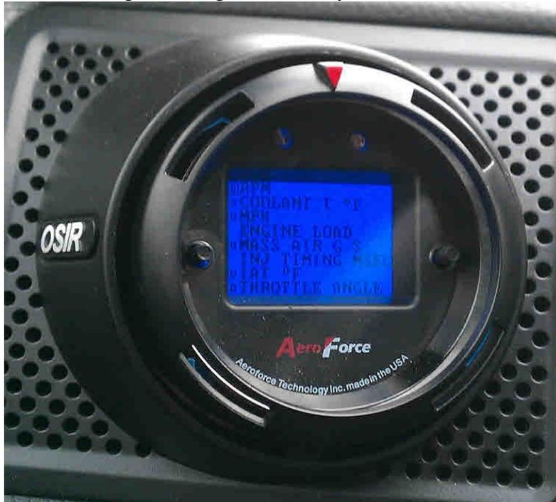
**2. Cyclic:** By selecting this, all items selected in **Parameters** will be shown. **Cyclic**, or better known as cyclic scan, allows you to choose up to 8 parameters that will be automatically toggled through without hitting any buttons. They will be displayed on the upper/lower field format used in normal scan mode.
