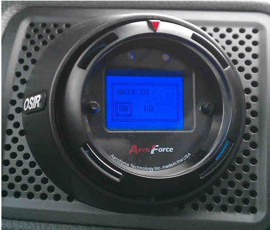
Make your selection by highlighting it and then pressing both buttons at the same time. After this step you will be taken back to normal **Scan** mode. The Annunciator will be active at this point. To turn it off go back in the main menu, toggle to “**Annunciator Off**” (this replaces the original selection titled “**Annunciator**”) and select. This will now go back to saying “**Annunciator**”.
