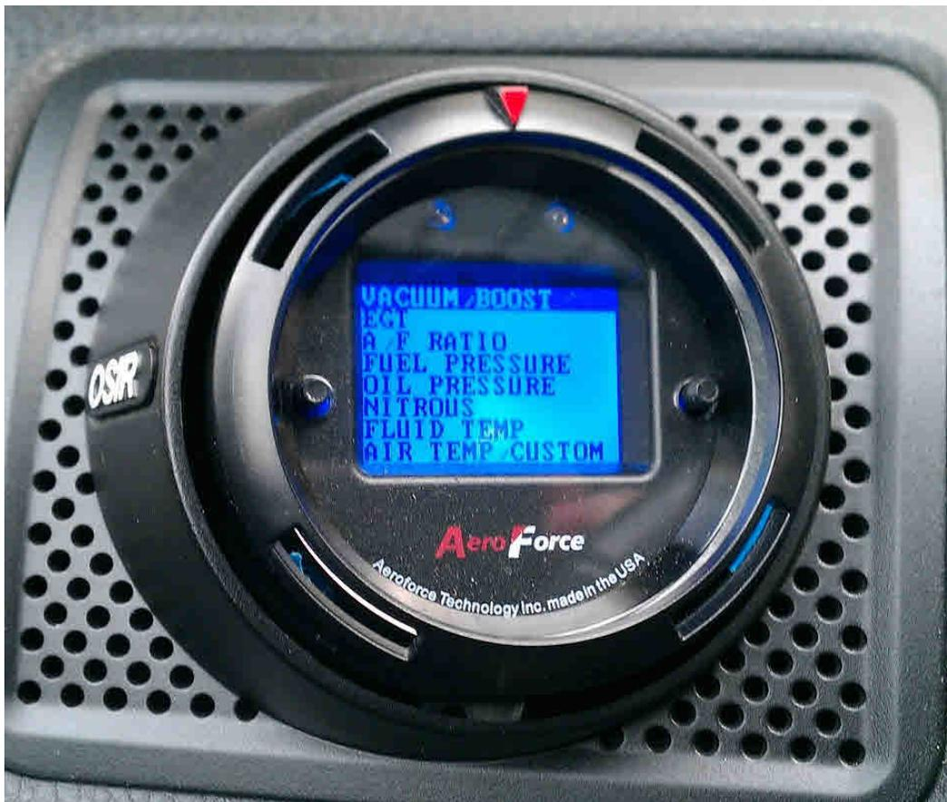
Toggle to the desired name and press both button. If you are using a temp sensor, select **Fluid Temp** or **Air Temp**, then select “no” if asked if you want a custom label. To enter a custom label choose “**Air Temp/Custom**”. You will then see this screen:
