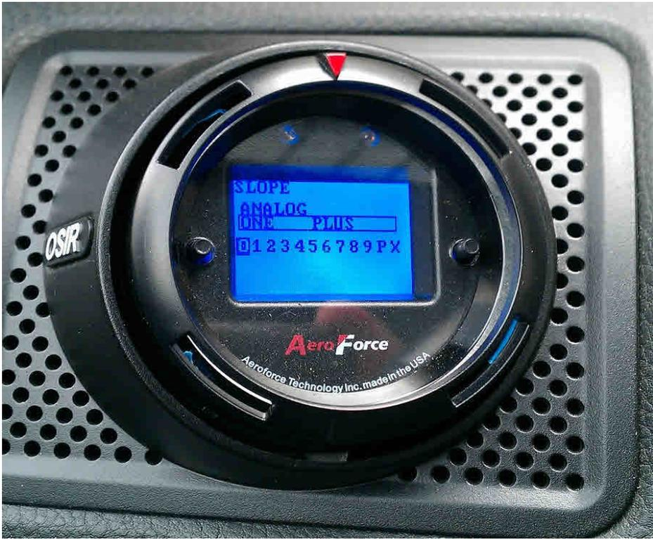
Toggle to the desired digit using the buttons, press both buttons to select. Repeat until slope is entered. To finish, toggle the “X” at the end and select it. You will be asked to confirm by pressing the right button. You will go to the intercept value entry screen. Repeat the process. Upon exiting, you will be asked if you want to choose or enter a name description:
