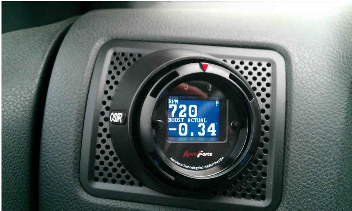
To select a menu option, momentarily press both buttons while on that selection. Once in a menu selection, if you are asked to choose between options, toggle to the option desired using the left and right button and press both buttons to select.
