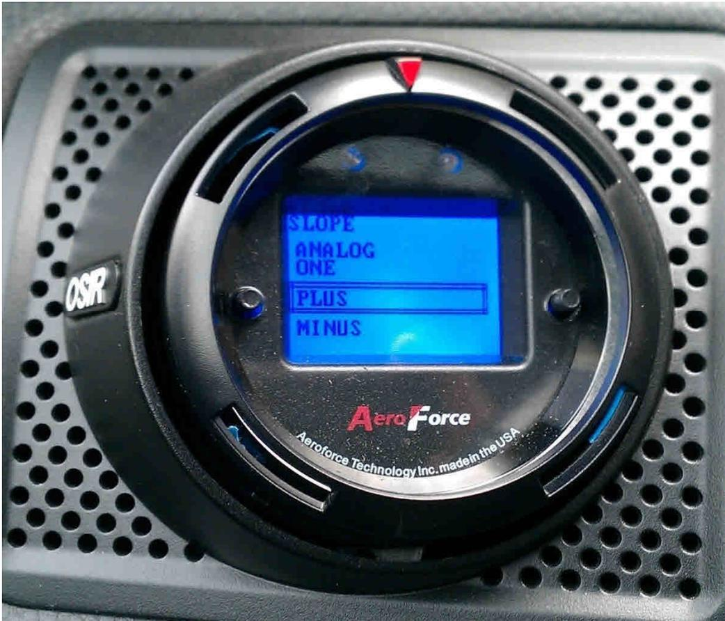
Using the buttons, toggle to the appropriate sign, then press both buttons to enter. You'll then go to the next screen and be asked to enter the value:
