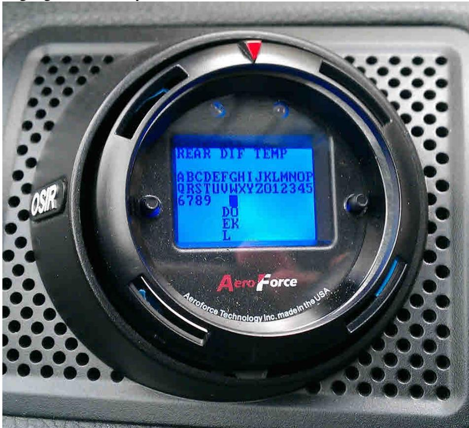
You will then toggle to the letters needed, selecting each by highlighting and pressing both buttons. The third to last spot is empty and is selected for a “space”. The second to last is to delete a mistaken entry, and the last, “Ok”, is to accept and exit.
