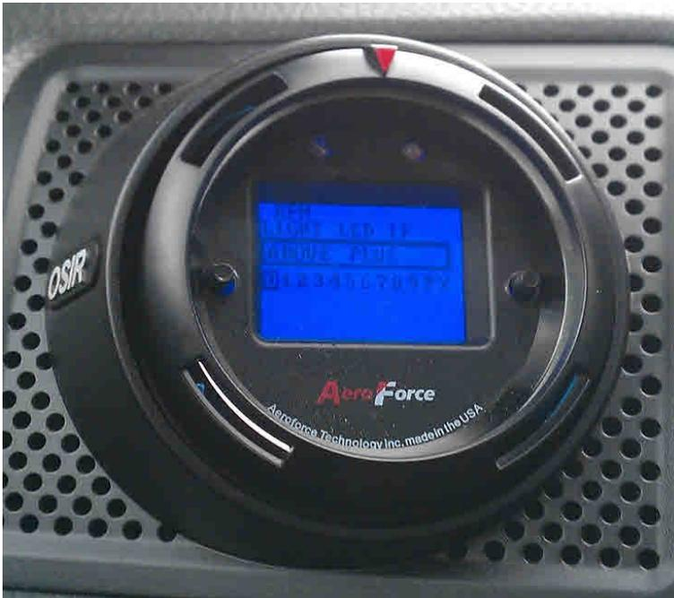
Finally it will ask for a rate, default being 1. This rate represents how many scans of displayed data before the annunciator will look at the monitored parameter(s). “1” is the fastest rate you can select. “4” would allow both parameters to update twice for each time the annunciator looks at its parameter. Slower changing parameters like temperatures can be monitored less often allowing the normal scan mode to update faster.
